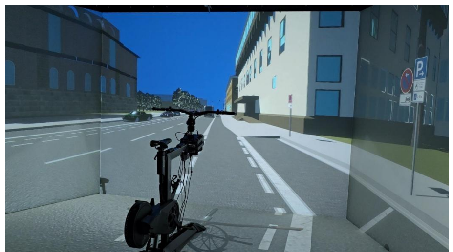
Figure 2: The physical simulator setup showing the multi-screen CAVE environment and the stationary fitness bike
