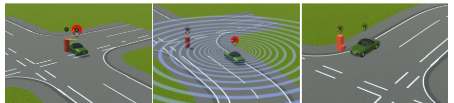
Fig 4: AEB system in work to avoid collision
