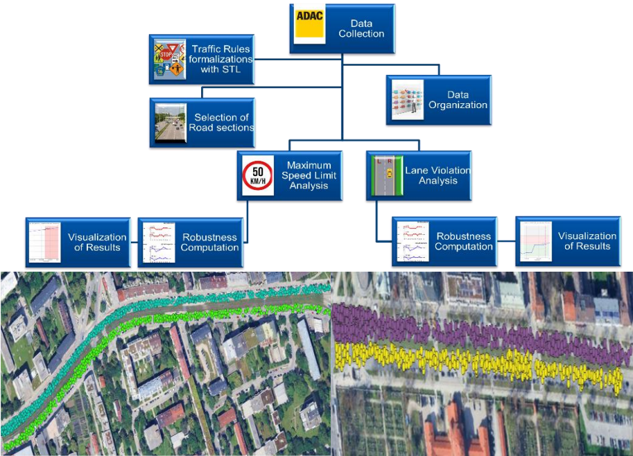
Figure 2: Overview of Methodology and road sections with highlighted dataset
