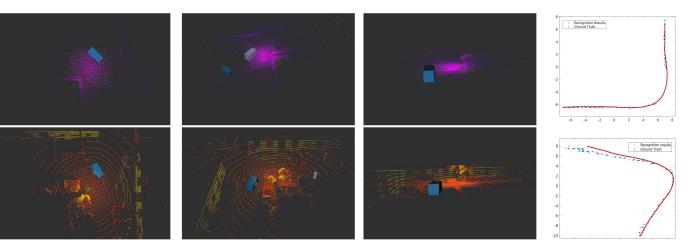
The differences in trajectories and inaccuracies in pose we just observed illustrate that continuous improvement is necessary. To address existing challenges and improve the reliability and applicability of digital twin models, we should explore alternative experimental configurations, algorithm enhancements, controller optimization, and the research of different scenarios as well as the time synchronization test.
