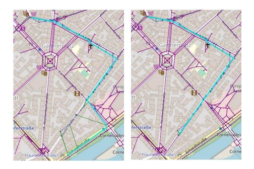
The processed network shows advantages in computational time as parts of the network are simplified. However, the accuracy was in the same range as the raw network, so the processed network is a good variant for this size of project area (see blue dots in figure on the left). For smaller areas, the raw network can be a good alternative as the computation time is less and the average distance error comparable (green dots in the figure on the left).
