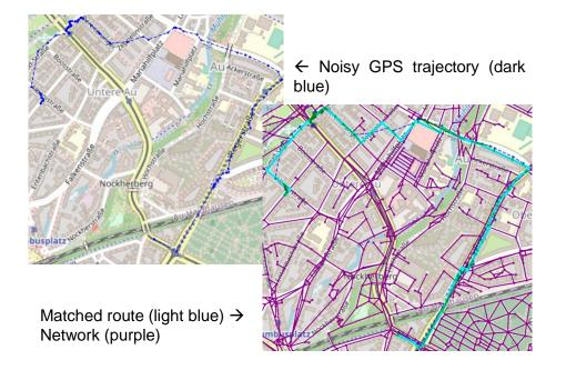
The algorithm needs a network of edges and nodes to match the GPS measurement on them. Therefore, a raw network (RN) is used including different types of layers for different modes based on OSM data. Secondly, a processed network (PN) is used where the basis of OSM data from whole Munich is simplified to reduce the number of edges in the network and to save computational time.
