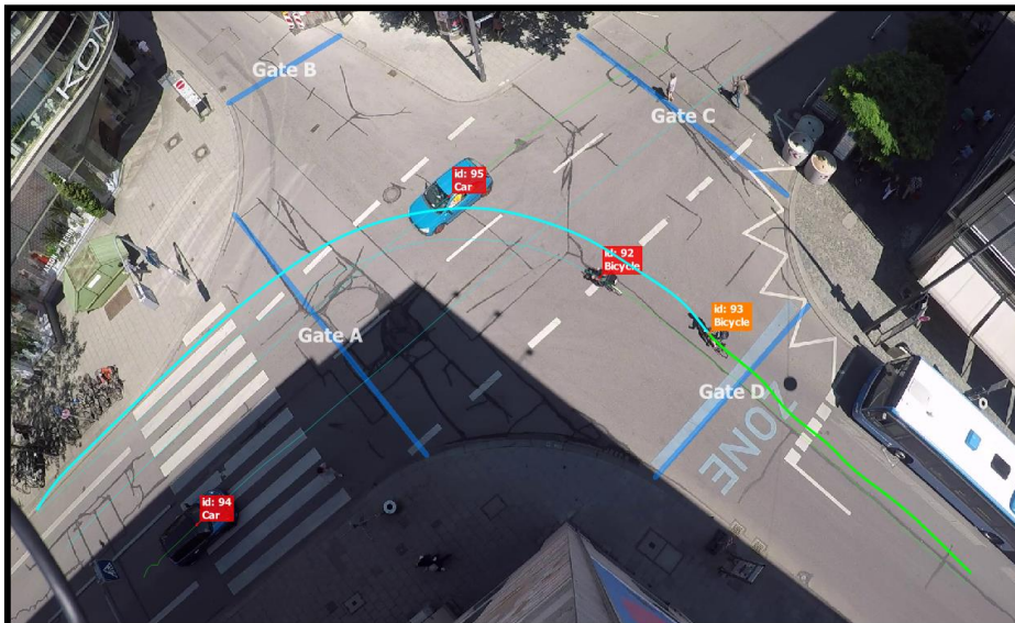
Fig. 1: Tracking of Traffic Participants with a Tracking Software (tracked trajectories are shown as colored lines)
