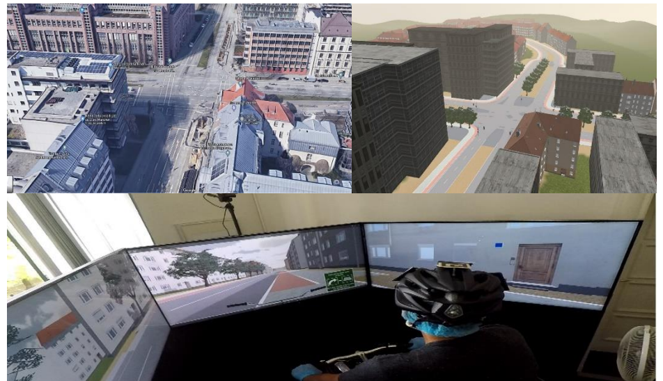
Fig. 1: Comparison of an intersection in the real world and in a simulation environment (top) and a participant while driving in a simulated traffic environment (bottom).
