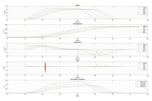
The EIDM (Enhanced Intelligent Driver Model) is selected as the original model to do the enhancement since it is an "intelligent" model with a crash-free characteristic. Besides, it has more realistic behaviour than the IDM (Intelligent Driver Model) at a critical situation.
