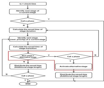
Figure.3 A new algorithm flow chart
