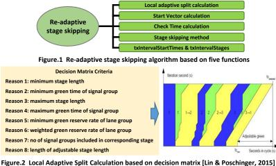
Figure.2 Local Adaptive Split Calculation based on decision matrix [Lin & Poschinger, 201
