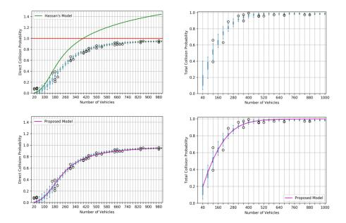
Extending upon Hassan and Vu's (2011) model, a new integrative analytical module was developed, which merges realistic vehicle mobility impacts and wireless channel characteristics. As a result, an integrative module was tested on urban scenarios, compared and validated with a widely used simulator, with the intention of proving its effectiveness of providing rich insights in the performance assessment of vehicular communication networks.
