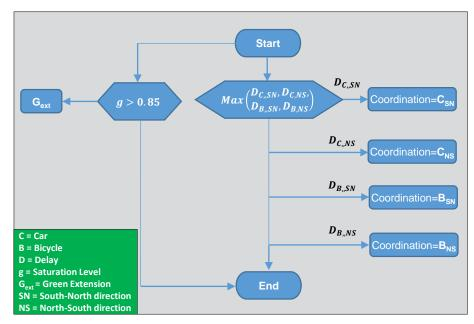
Fig.2 Optimum objective function as the algorithm of the new control strategy
