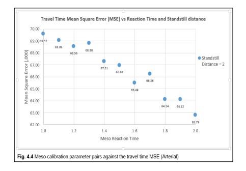
Microscopic Simulation of Arterial Road: The volume in the network were sensitive to changes in Wiedermann 99 car following model parameters. However, the travel time was not sensitive to the parameter changes.
