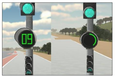
Figure 1: Two bicycle countdown timers tested in the simulator study: "seconds timer" (left) and "circle timer" (right)
