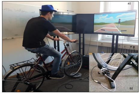
Figure 2: Bicycle simulator (a) and detail of the rear wheel fixed on a bicycle trainer (b).
