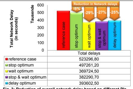
Fig. 3: Reduction of overall network delay based on different PIs
