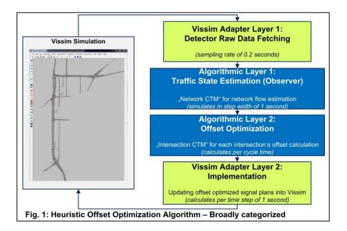
The broadly categorized methodology contains four major layers as shown in Fig. 1 which communicates in a hierarchal manner with Vissim Simulation. Network CTM is used to calculate network wide CFP based on stage recall detectors and without usage of system loop detectors (~160m to stop-line) which is considered necessary in SCOOT. The Network CTM builds an online traffic state estimator which can be used independently of an offset optimization algorithm.
