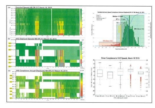
In the comparison of compliance data from a segment of the Autobahn 99 with the OR 217, the lowest speed of the German system starts mid-range in the Oregon system. The top speed for the OR 217 system is 50 mph or 80 km/h compared to 75 mph or 120 km/h for the A99 freeway in Munich. In the Oregon system, as the displayed speed increases, driver compliance becomes better. On the A99, drivers tend to drive increasingly faster than the speed limit, as the speed limit becomes higher.
