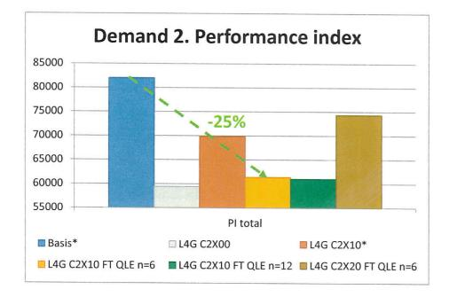
Successfully implemented queue length estimator and optimization algorithm for the speed recommendations have improved overall results.
