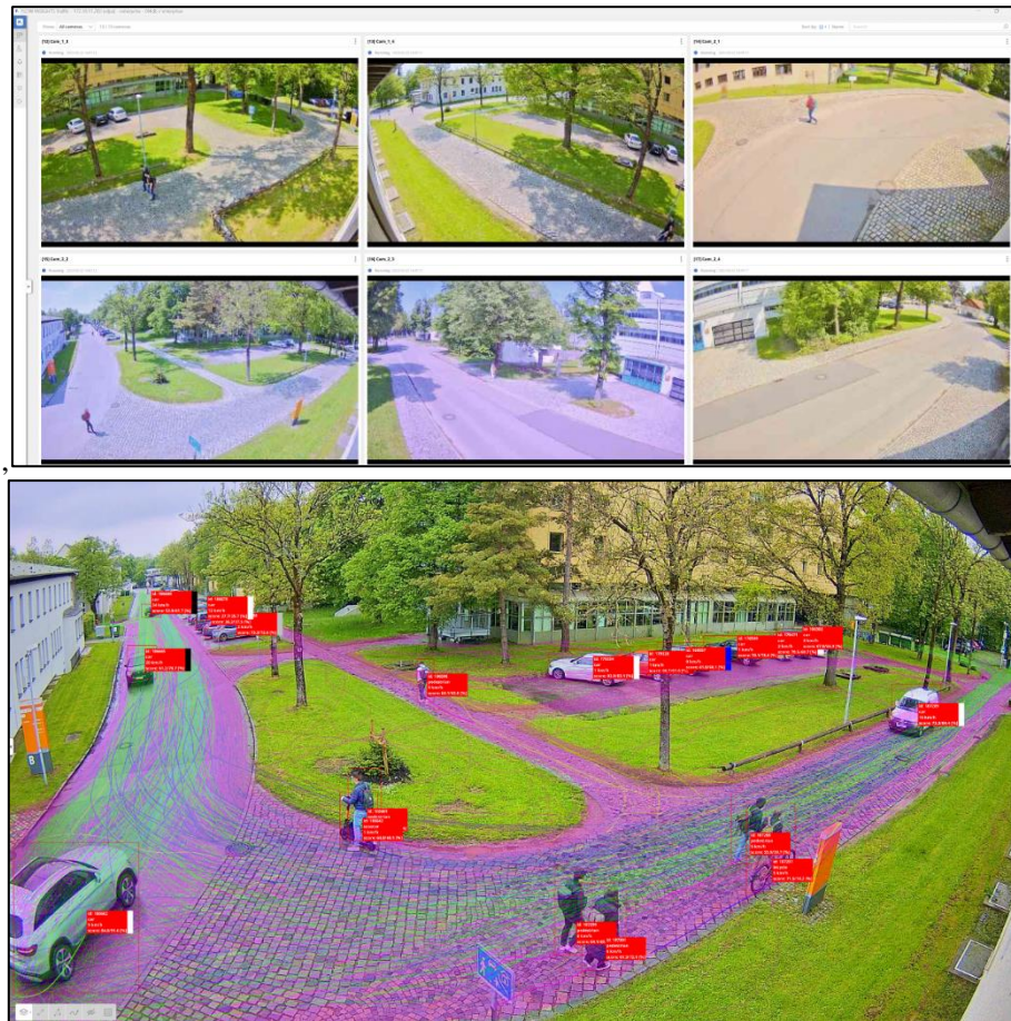
Figure 1: The traffic data collection system in the research project MORE
